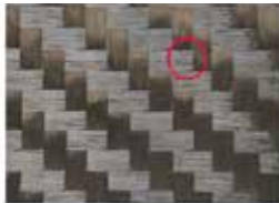
PrimeTex® 193 gsm, Twill 2/2, HS12K Open factor: 0.3%
